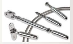
length and push it into the Quick-Connect fitting, and the one-way spring-loaded jaws lock it in place. Feeney offers a variety of fixed-end and tension-adjustment fittings, all made from 316 grade stainless steel and designed to accommodate <sup>1</sup>/8-inch-diameter 1x19 stainless cable. Prices range from \$16 to \$41 per fitting.
