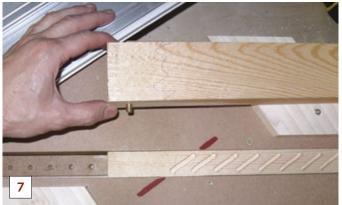
(5) is locked at the correct offset distance. The sliding router base travels between two stops (6) that limit the length of the flat-bottom mortises.
