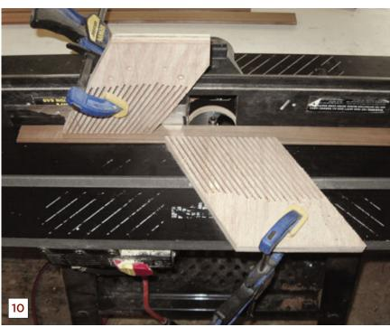
Reaming out the holes helped reduce any misalignment between the two pegboard strips, ensuring that the pin would drop into place without hanging up.
