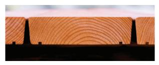
Premium Decking. Each board in the new Heritage Collection of 2x6 redwood decking is hand-picked and run through the planer at low speed to give it a refined finish, says the maker. The boards are milled with a crowned top surface, beveled edges, and drip channels that shed water. Prices start at \$1.75 per linear foot. The collection also includes two types of railings.
