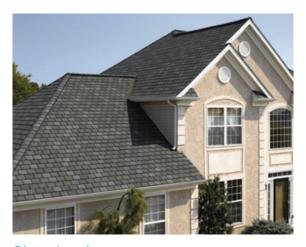
Slate Look. CertainTeed's Highland Slate is a single-layer fiberglass shingle that duplicates the texture and color of natural slate. The four-tab 18-by-36-inch shingles are rated for high-wind zones (an impact-resistant version is also available) and come in six colors. They cost about \$130 per square.
