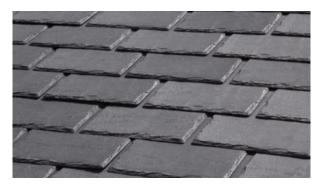
Recycled Roofing. Even up close, EcoStar's roofing tiles could easily be mistaken for weathered shakes or antique slate. But they're made of rubber, 80 percent of it recycled from post-industrial scrap. Seneca Shake and Majestic Slate tiles are UL-listed for fire resistance and Class 4 impact resistance. Each line offers 10 color choices and a variety of widths and thicknesses. Prices start at \$3 per square foot.
