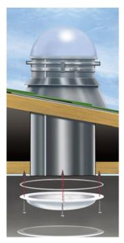
**Premium Tube** Light. SunPipe tube skylights feature clear acrylic top domes, industrial-grade galvanized-steel flashings, and aluminum pipes coated with a highly reflective silver lining. They're sold in 9-, 13-, and 21-inch pipe diameters. A basic 9-inch kit costs \$310.
