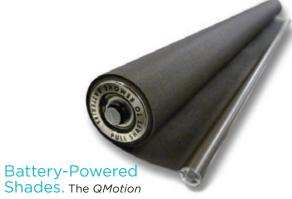
may look like a simple pull-down shade, but a motor and battery pack are concealed inside its roller tube. According to the maker, the roller's precision steel ball bearings are so effective at reducing friction, the unit can run for up to five years before the standard (D-size) alkaline batteries have to be replaced. The shade is made to order and comes in a wide range of colors and textures. Prices start at \$450.
