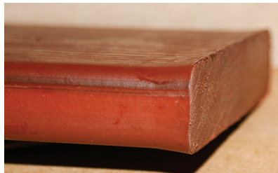
The ends on these capstock deck boards swelled because of water absorption in a lab environment.
