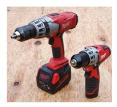
Milwaukee's subcompact drill/driver (right) is much smaller than the author's 18-volt lithium-ion hammer-drill (left) and weighs about 3<sup>1</sup>/<sub>2</sub> pounds less.
