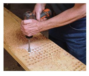
The author mounted a new Irwin <sup>3</sup>/4-inch Speedbor spade bit in each drill/driver, then counted the number of holes he could drill through 2-by Douglas fir per charge in high gear. He tested both of the batteries included with each tool.
