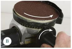
When it's outfitted with fresh 36-grit sandpaper, the Festool (A) is fast and smooth. Effective dust collection depends on correctly positioning a moveable brush by rotating an auxiliary handle; turning the handle clockwise rotates the brush counterclockwise (B). A quick-release lever (C) makes it easy to remove and adjust the Festool's extractor hood, but an inadvertent bump can knock everything out of alignment.
