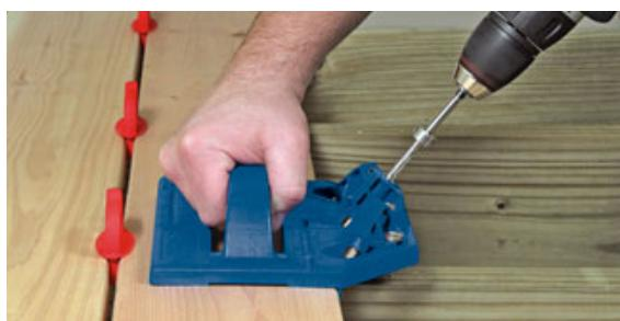
**Pocket Screws for Decks.** The company that pioneered the use of hidden fasteners now offers a jig that helps you fasten deck boards. The *Kreg Deck Jig* is compatible with any solid decking material between  $\frac{3}{4}$  inch and  $1\frac{1}{8}$  inches thick, though you need a minimum deck spacing of  $\frac{1}{4}$  inch to fasten the boards from both sides. A kit — the jig, spacer rings, a drill bit, and a drive bit — costs \$100 online.
