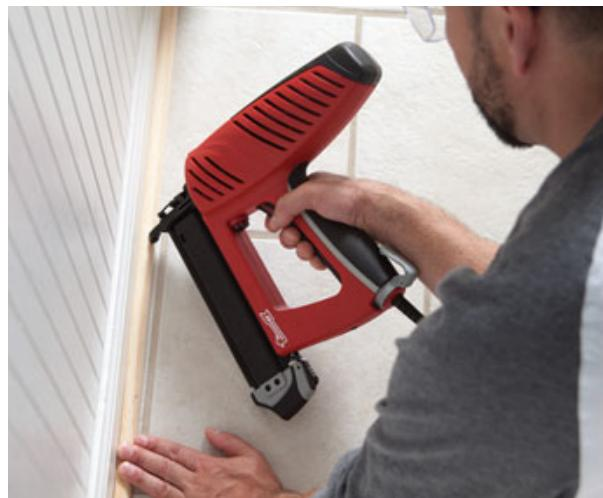
**Plug-in Brad Nailer.** If you're tired of lugging around a bulky compressor to power a tiny brad nailer, you might want to check out Arrow's new *EBN320 RED Professional Electric Brad Nail Gun*. The manufacturer claims that this tool can precisely drive 18-gauge brad nails up to 2 inches long. Its features include an easy jam-clearing mechanism, an LED guide light, and a rotating belt hook. It costs \$135.
