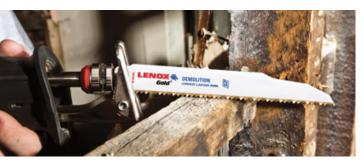
Improved Recip Blades. Lenox says its 72 demolition and wood-cutting reciprocating-saw blades now cut 25 percent faster than earlier models and last twice as long. According to the company, a change in the shape and pattern of the teeth reduces friction and helps the blades cut faster in nail-embedded wood. A five-pack of T2 blades costs \$14 to \$25, depending on the size and specification.
