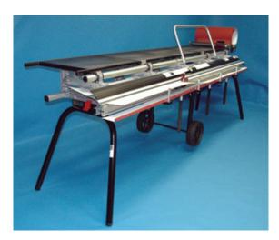
Big Brake. Aluminum fabricators who fly solo might appreciate the *Ultima Plus Alum-A-Brake*, which has a removable work table that pops off in five seconds, lightening the load by 20 pounds. Other features include a built-in track-mounted slitter and a slitter guide bar that eliminates the need to account for the offset. The 10-foot 6-inch brake costs about \$1,350; 7-foot 10-inch and 5-foot 11-inch versions are also available.
