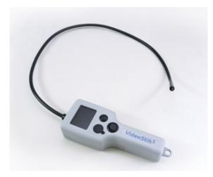
Affordable Inspection. With a price tag of just \$200, the VS36-10WD Video Scope may hasten the day when every remodeler has an inspection scope in his or her tool kit. Instead of an eyepiece, this scope has a full-color 2.5-inch LCD screen. It operates with a simple toggle switch. An RCA jack lets you connect it to an external monitor or a video recorder. The basic model comes with a 36-inch lighted shaft; a 72-inch shaft is also available.
