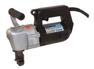
Nastier Nibbler. Kett recently upgraded its AN3000 nibbler. The new and improved model -AN3500 — has a 6-amp electric motor and can chew through 10-gauge cold rolled steel or 12-gauge stainless at a rate of 90 inches per minute, the maker says. Thanks to a redesigned plunger, die holder, and punch, it also operates more smoothly and should last longer than its predecessor, the company says. It costs \$188.
