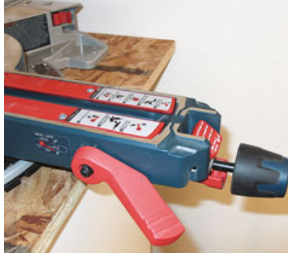
Readily accessible finger-operated features like the up-front bevel control (left) and quick-release sliding fence (right) make for easy tool-free adjustments.
