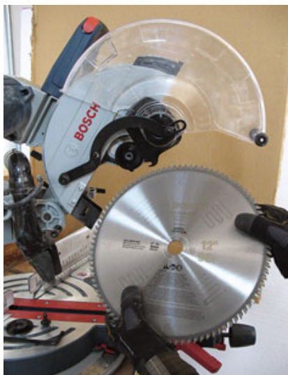
The blade guard on the Bosch gets out of the way easily when it's time to change blades.
