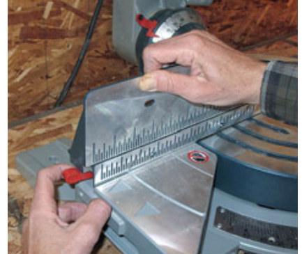
Readily accessible finger-operated features like the up-front bevel control (left) and quick-release sliding fence (right) make for easy tool-free adjustments.
