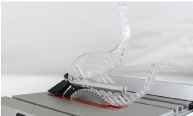
Each half of the plastic blade guard operates independently. One side or both sides can be tilted up and out of the way. For tricky operations, the entire assembly removes with the flip of a lever.
