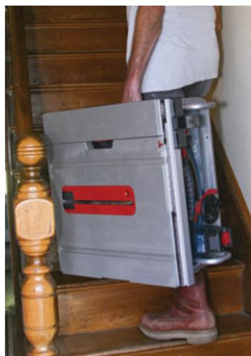
A rubber handle on the side of the steel roll cage makes it easier to maneuver the GTS1031 through tight spaces.
