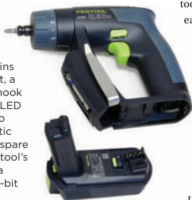
The Centrotec quick-change chuck accepts Festool's Centrotec bits and bit holders. The Centrotec BH 60MM magnetic bit holder (shown here) is included with the kit, and drives standard hex-shank insert bits.
