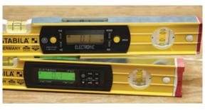
The Stabila Type 196E Tech (top) is being replaced by the IP65 Tech (bottom). New features include a backlight for much easier viewing in dim light, better seals, and bouncier removable end caps.
