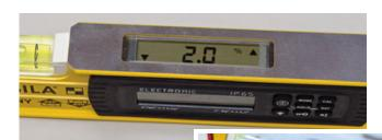
The level can read slopes in a variety of formats. Here, it's indicating a common 2 percent drainage slope (above) and a 4/12 roof pitch (right).
