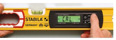
The display is typically calibrated by holding the level against a vertical surface, leveling it visually with the center vial, and then pressing the CAL button twice.
