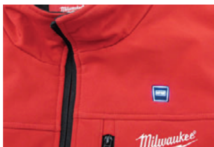
The "M12" logo on the lapel doubles as the on/off button for the heating unit. It changes color — white, red, blue — to indicate the temperature setting.
