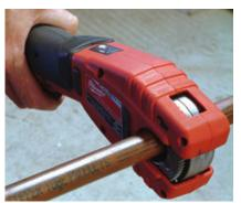
The copper-tubing cutter must be open to grab or release a pipe. To open it you move the control switch in front of the trigger to the far right and then pull the trigger (top). The window makes it easy to align the cutting wheel with the cutline and can be lit by pressing the white button, which also lights the LED battery gauge (center). To make a cut, you flip the control switch to the far left and squeeze the trigger, which spins the cutting wheel around the pipe (above).
