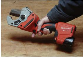
Designed to fit into tight spots, the PVC shear cuts up to 2-inch Schedule 40 PVC pipe (top). To cut, you push the lock-off button with the base of your forefinger while squeezing the rear trigger with your middle finger (above). This also lights up the LED battery gauge for about two seconds. Pulling the front trigger alone springs the blade open.
