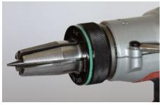
To join Uponor's AquaPEX tubing to its ProPEX fittings, you slip a ring over the end of the tubing, stretch the ring and tubing with an expansion tool, then slip them over the fitting and let them shrink to a leak-free fit. The M12 ProPEX expansion tool makes the job easy and fits into tight spaces (left). The expander heads simply thread onto the frame (top right). When you pull the tool's trigger, the jaws repeatedly open and close as the head rotates incrementally (above right).
