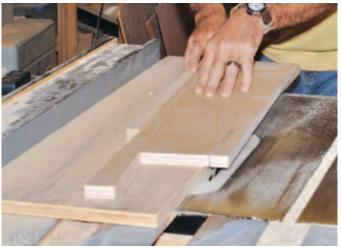
**1.** To safely cut the tapered <sup>3</sup>/4-inch plywood panels, I made a plywood sled for the table saw and used the drop from the first angled cut as a spacer for cutting the remaining edges.
