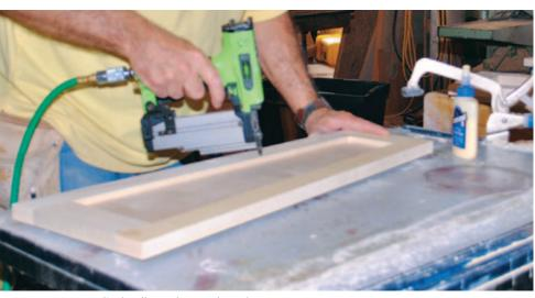
**3.** I applied yellow glue to the rabbets, dropped the panels in place, and secured them with headless pins while the glue dried.
