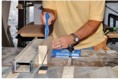
**1.** To make the cap, I glued up a 2-inch-thick block using two lengths of 4/4 poplar. I ripped the stock to equal half the width of the top of the post plus another  $^{1}/_{2}$  inch for the overhang. I then ripped a 35-degree bevel angle on one surface.
