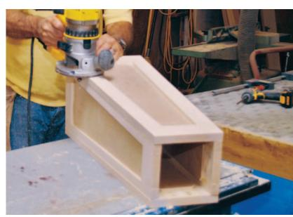
**3.** Setting the two wider frames slightly proud of the two narrower frames made it easier to flush-trim the joints with a router after the glue dried; this resulted in better-looking joints. I cleaned up the 26-inch-high assembly with a random-orbit sander and 120-grit paper.
