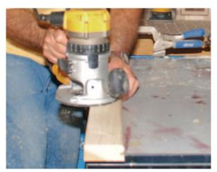
**1.** I made the trim that hides the joint between the two paneled sections with a large beading bit mounted in a handheld router.
