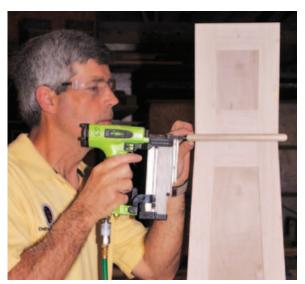
**3.** I ran the trim through a planer to clean up the surface, then glued and pinned it in place.
