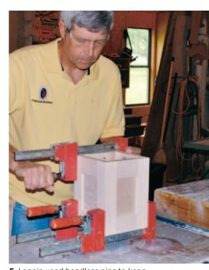
**5.** I again used headless pins to keep the panels aligned as I clamped them together.
