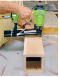
1. Next I made the column that would reinforce the panel assemblies. I used <sup>3</sup>/4-inch plywood and sized the column to fit snugly — keeping in mind that, because the plywood panels extend <sup>3</sup>/8 inch past the inside of their frames, the overall clearance inside the upper assembly was reduced by <sup>3</sup>/4 inch.
