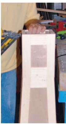
**3.** I used the story pole to make sure the top paneled section would end up flush with the top of the inner column.
