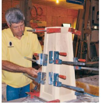
**2.** The clamps provide the pressure, while the headless pins keep the panels aligned.
