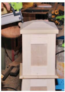
**3.** I fastened the cap to the post with glue and headless pins.
