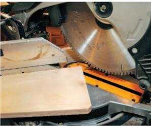
**2.** Instead of squaring the corners of my rabbet in the back of the frame with a chisel, I clipped the corners of each plywood panel with the miter saw.
