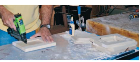
**4.** While the tapered glue-up was drying, I made the four rectangular panels for the 9-inch-high upper assembly in the same way.
