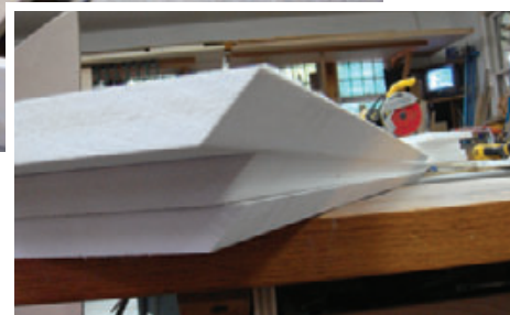
Figure 4. The MDF template is screwed to the PVC blanks (left), which are then routed with a large 45-degree chamfer bit (above), leaving a crisp mitered edge (right).
