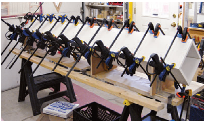
Figure 5. Biscuits (far left) ensure accurate alignment as the half-columns are glued together; note the squaring blocks (left). Plywood gluing cradles (below left), accurately sized to match the tapering columns, make it easy to place the clamps. Though they are gluing a single corner, the authors have placed clamps on all four sides to keep things square (below).
