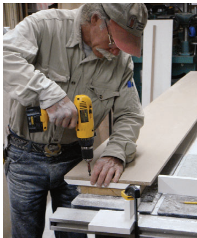
Figure 4. The MDF template is screwed to the PVC blanks (left), which are then routed with a large 45-degree chamfer bit (above), leaving a crisp mitered edge (right).
