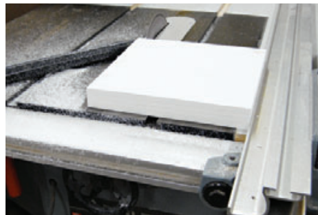
Figure 6. While the cement on the columns was drying, the authors set up another gluing station for the caps and bases, which they laminated out of two pieces of \frac{3}{4} -inch PVC (far left and left), then trimmed to final size on the table saw (above).
