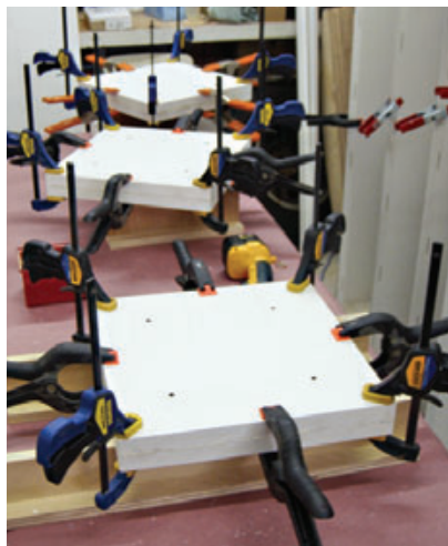
Figure 6. While the cement on the columns was drying, the authors set up another gluing station for the caps and bases, which they laminated out of two pieces of \frac{3}{4} -inch PVC (far left and left), then trimmed to final size on the table saw (above).
