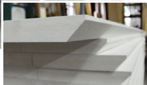
Figure 3. Before final routing of the edges, the authors trimmed the PVC blanks to within \frac{1}{16} inch of the cut line (above left), then wasted most of the miter material on the table saw (above right), leaving only a narrow vertical band to safely ride against the fence (right).
