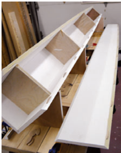
Figure 5. Biscuits (far left) ensure accurate alignment as the half-columns are glued together; note the squaring blocks (left). Plywood gluing cradles (below left), accurately sized to match the tapering columns, make it easy to place the clamps. Though they are gluing a single corner, the authors have placed clamps on all four sides to keep things square (below).
