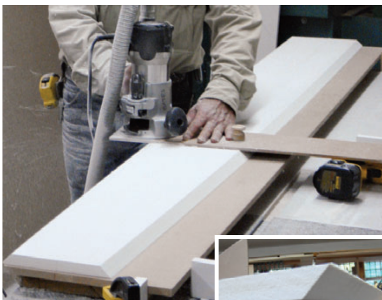
Figure 4. The MDF template is screwed to the PVC blanks (left), which are then routed with a large 45-degree chamfer bit (above), leaving a crisp mitered edge (right).
