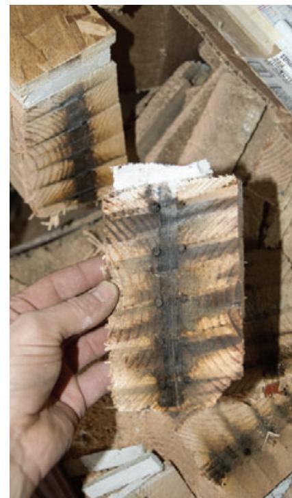
The author used a stopwatch to time cuts through the test planks. A blade was considered dead when it took more than 37.5 seconds per cut; by that point, most blades could barely get through and were hot enough to char the wood.
