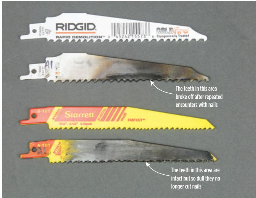
Tooth size alone is not a good predictor of longevity. The widely spaced teeth of the Ridgid blade (at top) cut quickly at first but were prone to snagging on nails. The more tightly spaced teeth of the Starrett didn't lose teeth to shock, but friction and heat eventually wore them down.
