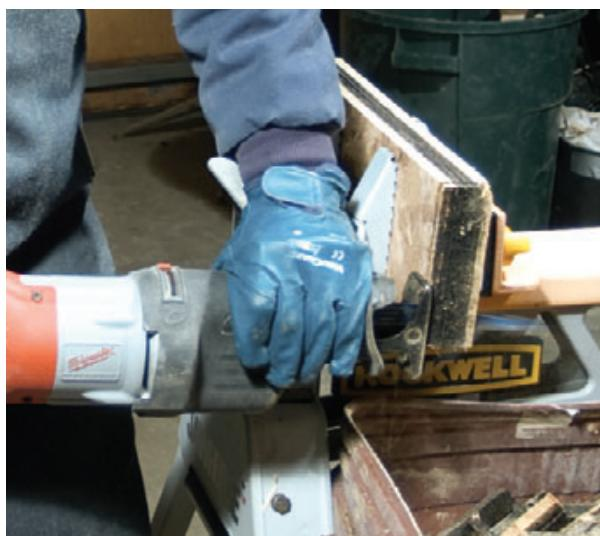
The author tested for resistance to abrasion by sawing through shingles sandwiched between pieces of OSB (left). As was typical of the bimetal blades tested, the teeth at the center of this model (shown below after 22 cuts) were completely worn away. Only the carbide-tooth blades survived for long in shingles.
