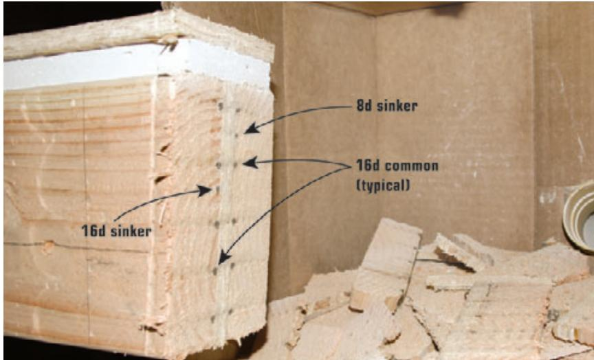
The test plank consisted of a piece of OSB sandwiched between 2x6s and capped with drywall and more OSB. The central piece of OSB was flanked by 12 rows of nails — so the recip blade had to cut 12 nails each time it went through the plank.
