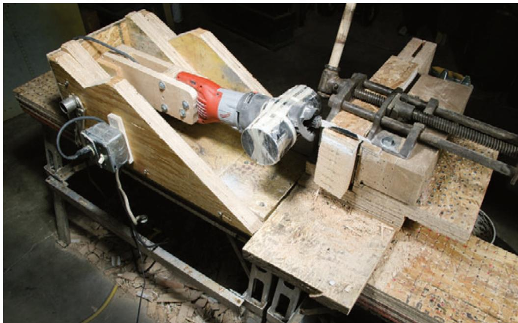
For timed cuts, a plank was clamped into a test rig and cut with a saw attached to a pivot arm. The nose of the tool was weighted to provide downward pressure — approximately 23 pounds at the blade.
