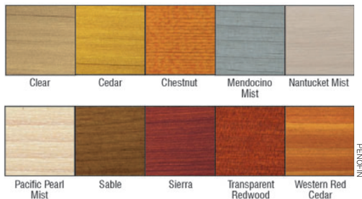
Figure 2. Toners and semi-transparent and solid stains are available from most manufacturers in a wide range of colors. Every wood species takes pigments differently, and while color charts can provide some guidance, don't rely on them. Doing your own color tests on sample boards is the most reliable approach. Toners allow the most grain to show while semi-transparent stains allow less.
