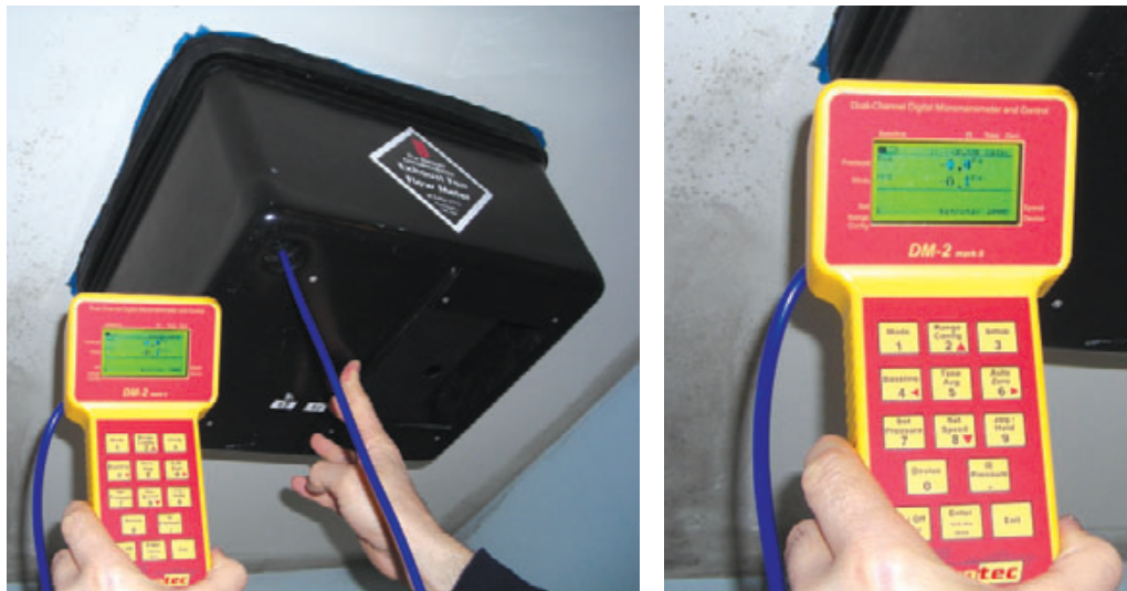
Figure 2. The author checked the airflow of the two fans using a duct hood and a manometer. He found that the fans were working at only about 60 percent of their rated 70-cfm capacity.
