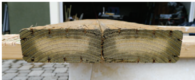
Figure 2. Pressure treatment doesn't force the preservatives all the way into the wood. That's why additional steps are required to keep water from soaking in.
