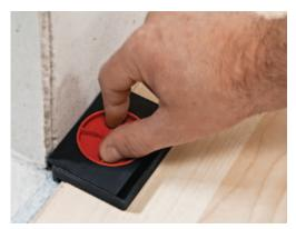
Adjustable Spacer. The AV2 Flooring Spacer might spare you the hassle of hauling a bucketful of shims from job to job. The business-card-sized spacer block adjusts with the turn of a dial from 5 to 20 mm (<sup>3</sup>/16 inch to <sup>13</sup>/16 inch) to create a precise expansion joint between the floor and the wall, or to compensate for a wavy sole plate. To remove the spacer, you just turn the dial again to release the pressure. A four-pack costs about \$10.
