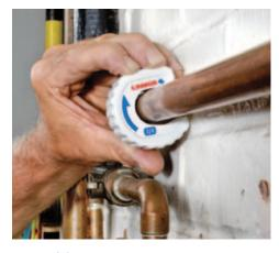
Knuckle Saver. Lenox says its *Tight* Space Tubing Cutter is easier to use than a typical mini cutter and requires only ½ inch clearance. (It's not adjustable, however, so you'll probably have to buy more than one.) It has stainless steel cutting wheels and a cast aluminum grip. A kit holding all three sizes — ½ inch, 3/4 inch, and 1 inch — costs about \$60.
