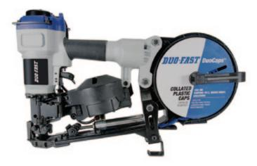
Double-Duty Cap Nailer. Duo-Fast's *DF175-CN* fastens synthetic roofing underlayment and felt quickly, says the maker, and — unlike other cap nailers — uses standard (120-count) coil roofing nails to secure the caps. To convert to nail-only fastening, the user simply pushes a button to shut off the cap feed. The tool has a tool-less adjustable depth-of-drive and a quick-clear nose. It drives nails from <sup>7</sup>/<sub>8</sub> inch to 1<sup>3</sup>/<sub>4</sub> inches and costs \$450.
