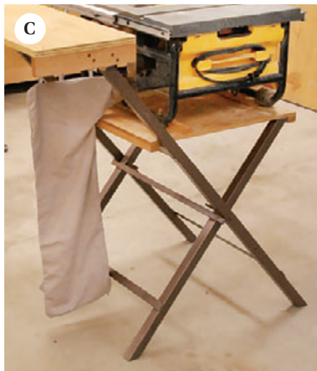
Figure 6. To haul long moldings or conduit, the author fabricated mini racks for his truck rack from a few sections of scrap metal (A). He first joined lengths of 1/2-inch by 1-inch stock to 1-inch-diameter steel tubing, then attached 1/4-inch band iron to the crosspieces to make the uprights (B). The fold-up table saw stand (C) was built from surplus 1 1/4-inch square tubing, while the tailgate bracket was also fashioned from scrap metal angle (D).
