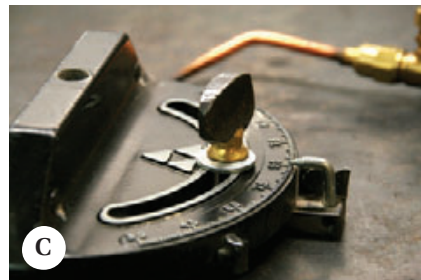
Figure 3. The author uses an oxyacetylene torch when working with dissimilar metals or making small repairs (A). Here, for example, he braze welds a new brass thumb screw to the existing steel bolt of his damaged miter gauge (B); a filler rod supplies the metal that joins the two components together (C).
