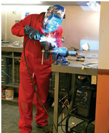
Figure 2. MIG wire feed welders are well-suited for thinner materials and indoor work. The wire and shielding gas feed through a relatively short (about 10 feet) hose, so the machine can't be placed too far away from the work.
