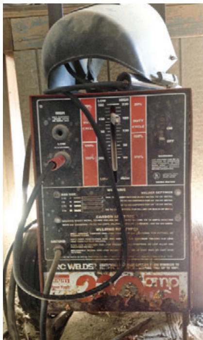
Figure 1. Stick welders are often used with thicker metals and for outdoor work. To protect the weld puddle from contaminants in the atmosphere, electrode rods are typically coated with a flux that creates a shielding gas when it burns. The author's vintage unit (shown) is slow but usable.
