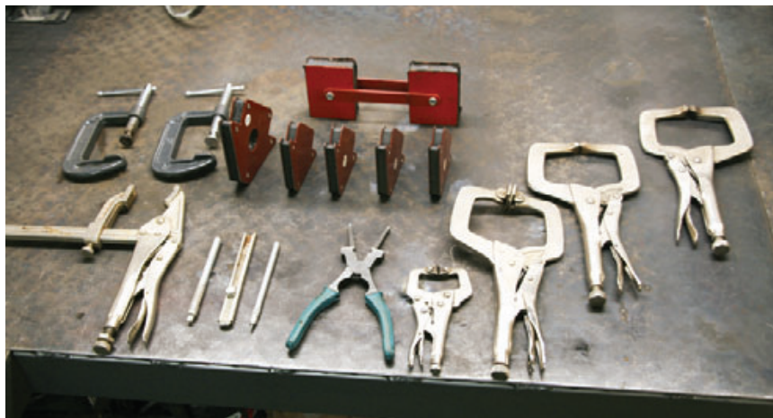
Figure 5. An assortment of clamps and magnetic welding holders is handy for holding metal parts square to each other while they're being welded together.
