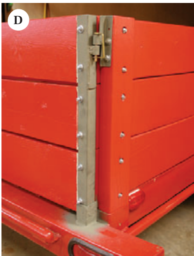
Figure 6. To haul long moldings or conduit, the author fabricated mini racks for his truck rack from a few sections of scrap metal (A). He first joined lengths of 1/2-inch by 1-inch stock to 1-inch-diameter steel tubing, then attached 1/4-inch band iron to the crosspieces to make the uprights (B). The fold-up table saw stand (C) was built from surplus 1 1/4-inch square tubing, while the tailgate bracket was also fashioned from scrap metal angle (D).
