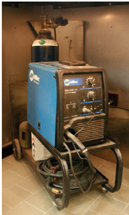
Figure 2. MIG wire feed welders are well-suited for thinner materials and indoor work. The wire and shielding gas feed through a relatively short (about 10 feet) hose, so the machine can't be placed too far away from the work.
