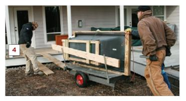
The design was determined in part by the scrap metal that was available in the recycle area of my local salvage yard. I used several pieces of 2-inch by 4-inch steel tubing with <sup>1</sup>/<sub>16</sub>-inch-thick walls to make the cart's frame. The 26-inch-long crosspieces are supported by 60-inch-long stringers, one of which I positioned on the flat when
