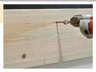
takes a  $\frac{5}{16}$ -inch hex driver, but sports the same tip design as the SDWS to eliminate the need for pre-drilling.
