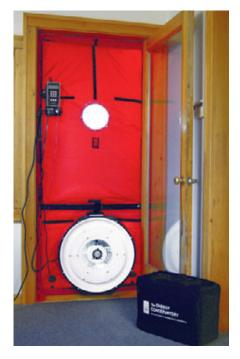
Ready-to-Go Blower Door. The *Minneapolis Blower Door* comes equipped with everything needed to measure airtightness or diagnose air-leakage problems, says the manufacturer. In addition to a lightweight injection-molded fan, the standard Model 3 kit includes analysis software, communication cables, a "Cruise Control" feature that lets the operator maintain consistent building pressure without a computer, a nylon panel, and an aluminum frame that fits an 8-foot-tall door. It costs \$2,500.
