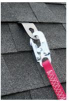
Long-Term Fall Protection. The key to the HitchClip Fall Arrest System is a 4.4-ounce anchoring clip that attaches to the roof framing with just four 16d (or equivalent) fasteners. Its compact size — 2 inches by 11 inches — means a worker can carry several in a toolbelt and install them as needed, says the maker. To make future roof access safer and
