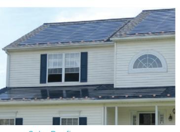
**Solar Roofing**. *Apollo* is a low-profile photovoltaic array that can be installed along with the shingles by a certified roofing contractor. It can also be set up on existing roofs. According to the manufacturer, the high-efficiency polycrystalline cells can produce 12 watts per square foot. The array is designed to be incorporated into asphalt shingle roofs with a minimum 4/12 pitch. Contractor's costs range from \$0.75 to \$1.50 per watt.
