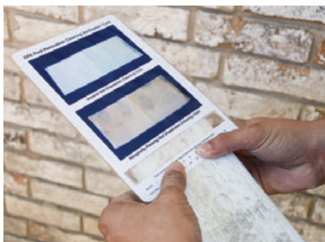
LeadCheck swabs (left) can indicate whether lead is present but can't determine the exact amount. After vacuuming, a verification card and handwipes are used to confirm that surfaces meet EPA standards (right).
