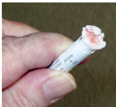
LeadCheck swabs (left) can indicate whether lead is present but can't determine the exact amount. After vacuuming, a verification card and handwipes are used to confirm that surfaces meet EPA standards (right).
