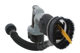
Dust-Catcher. The SawBuddie is a flexible rubber shroud — lined with bristles — that attaches to a recip saw. According to the maker, it captures as much as 99 percent of the dust generated by the saw without obstructing the operator's view of the cut line. When attached to a certified HEPA vacuum, it complies with RRP guidelines as a point-of-origin dust control system, the company says. It fits a variety of saws and costs \$80. An 18-inch-long hose adapter is available for \$20.
