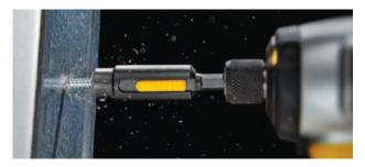
No-Clog Nut Driver. Removing metal shavings from a magnetized driver bit has never been an easy task — until now. DeWalt's *Cleanable Nut Driver* has a thumb slide that allows the user to push the magnet above the edges of the socket and simply wipe off the debris. It comes in five socket sizes (1/4 inch, 5/16 inch, 3/8 inch, 7/16 inch, and 1/2 inch), all of which have a 1/4-inch quick-release hex shank. Prices range from \$6 to \$11.
