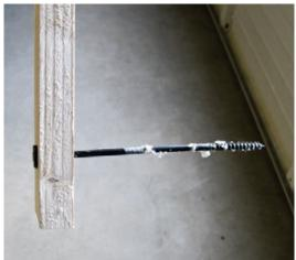
FastenMaster uses a highstrength steel for its fasteners, evidenced by the near perfect condition of many of the screws in the test (far left). On a few occasions when the strapping did not split or pull through, the screw showed only a slight bend (near left).
