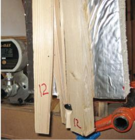
The strapping in this sample (far left) has crushed the foam, which offers little resistance. Note that the tops of the two layers of foam were flush at the start. In another test (near left), the wood has split and the fastener rotated at maximum load.
