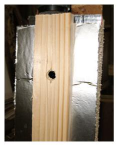
This sample is in position to be tested, with the head of the screw just proud of the strapping surface (left). As the force is applied, well beyond the yield point, the strapping begins to pull through as the screw rotates slightly (center). At maximum load, the head has pulled halfway through the strapping (right).
