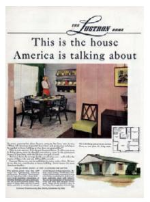
the outside. The space-saving design included interior pocket doors, built-in cabinets, and an innovative whole-house radiant heating system that warmed the living space by circulating 140°F air through a shallow plenum above the steel ceiling. Exteriors came in four colors — Surf Blue, Maize Yellow, Desert Tan, or Dove Gray — with white trim and dark gray roofing.
