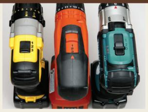
Three-speed trannies. The DeWalt, Hilti, and Makita (left to right) have a three-speed — rather than the usual two-speed — transmission. Makita's extra gear adds a second low-speed option for drilling big holes and other high-torque applications, while DeWalt's and Hilti's add a second high-speed option for less demanding applications like small-diameter drilling in metal.
