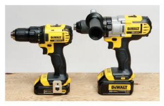
Full-size 18-volt drill/drivers can be significantly bigger and more powerful than their compact 18-volt counterparts. For instance, DeWalt recommends using auger bits up to 1<sup>1</sup>/<sub>4</sub> inches and hole saws up to 4 inches in diameter with its premium 20V Max (right), but the numbers drop to <sup>7</sup>/<sub>8</sub> inches and 2 inches, respectively, for its compact 20V Max (left). That's why most compacts don't have side handles.
