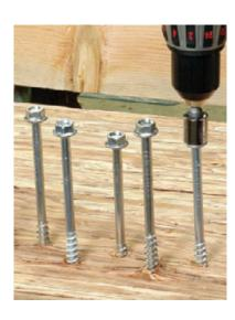
To size up the balance between maximum torque and overload protection, the author drove four 1/2-inch by 8-inch Spax lags as deep as possible into a PSL beam with each tool, then compared the average depth of penetration.
