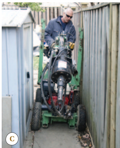
Figure 6. The author's small rig excels at going places larger pile-driving equipment can't (A, B, C). When the machine won't fit into a tight area, the drive head can be mounted on a portable bracket that bolts to the structure (D).
