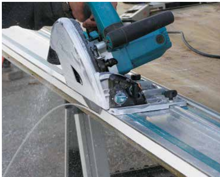
Figure 6. Instead of PVC trim boards, the author buys PVC in 4x8 sheets, then quickly and accurately rips his trim to the exact size needed with his track saw.
