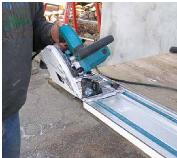
Figure 1. When you're making bevel cuts with the Makita SP6000K, a tab in the base of the saw engages with the track, which prevents the saw from tipping.
