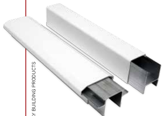
Figure 6. Vinyl rails are typically reinforced with internal aluminum channel, allowing spans of up to 12 feet.
