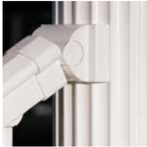
Figure 9. AFco's ( afco-ind.com ) aluminum stair railings are available with adjustable post brackets that pivot to accommodate stair angles between 0 and 36 degrees. The brackets are available to fit their fluted columns (above) as well as standard square posts (right).
