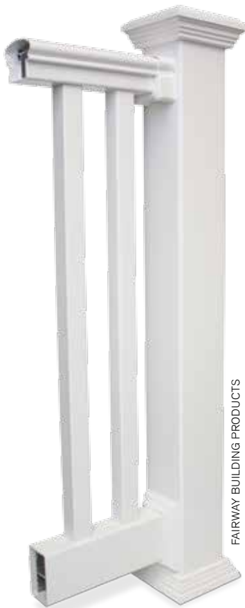
Figure 5. Fairway Building Products' Contour ( fairwaybuilding.com ) one-piece vinyl top and bottom railings are reinforced with aluminum inserts (left). The mounting brackets have vinyl covers that slide into place over the brackets, concealing the bracket fasteners but creating a rather bulky profile (above).
