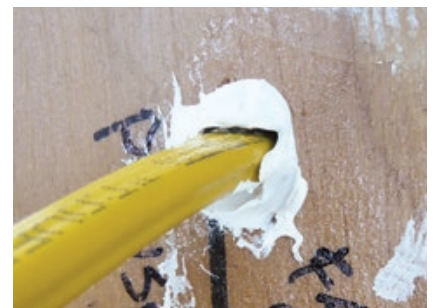
Figure 3. Caulks that failed the wire-movement tests typically remained bonded to the plywood but separated visibly from the outer sheathing of the cable.
