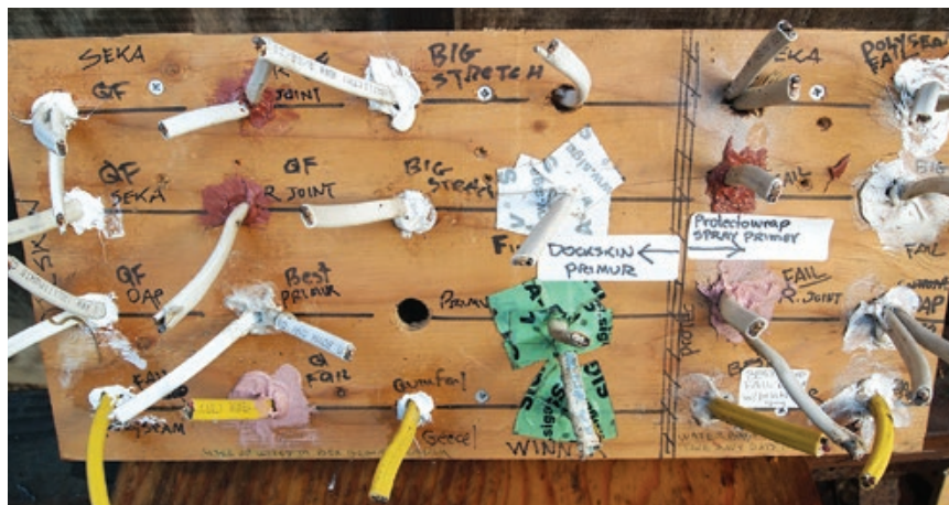
Figure 1. The gas-filled bubbles that give foam its cellular structure are durable if not stressed. But when pipes and wires air-sealed with canned foam are forcibly moved, these bubbles are easily torn apart.
