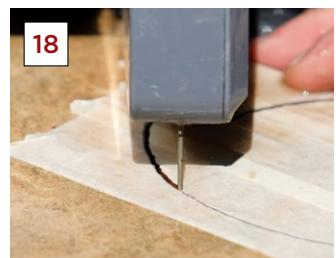
but in my opinion, they are not well-suited for production cutting of these materials. I use a ring saw when I need to make a large number of irregular cuts in relatively soft materials, but for most irregular cutting, I prefer to use a conventional wet saw.
