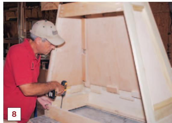
cleats that conformed to the slope of the hood (5), and a stretcher was placed between the tops of the side panels.
