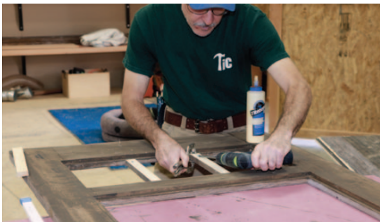
Figure 3. The author used 5/4-inch stock for the frames, and assembled the stiles and rails with Domino tenons (far left). The panels fit into 1/2-inch by 1/2-inch rabbets routed in the frames (left). Muntins at the top of the doors give the upper panes the look of divided lights (below).
