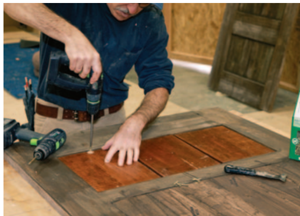
Figure 4. The panel edges were profiled with a raised panel cutter mounted on a router table (above). While fastening the panels to the frames, the author used his story pole to avoid placing screws where the doors would be cut (above right). The upper panels were made of Douglas fir, which the author stained before installation (right).
