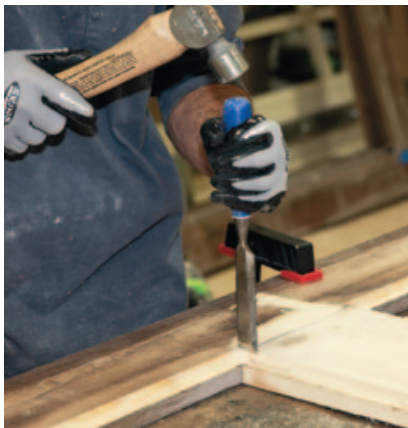
Figure 3. The author used 5/4-inch stock for the frames, and assembled the stiles and rails with Domino tenons (far left). The panels fit into 1/2-inch by 1/2-inch rabbets routed in the frames (left). Muntins at the top of the doors give the upper panes the look of divided lights (below).
