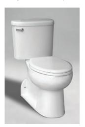
accommodate a drain pipe. The gravity-only flushing system uses just 1.28 gallons per flush: clogging problems are addressed with an oversized 3.15-inch trapway and a 3-inch flush valve. The chairheight ADA-compliant bowl is elongated and includes a soft-close seat, and the inside of the bowl has an antimicrobial surface. The toilet costs \$465.
