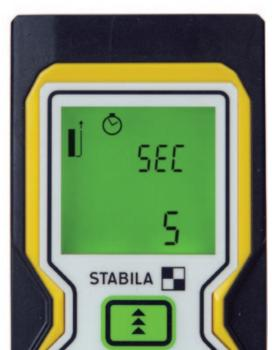
Timers. Six of the lasers have a programmable timer that delays the shot after you press the measure button. Because you can press then aim (rather than having to press the button while trying to keep the beam on the target) it's much easier to aim the beam precisely in an awkward position or at long distances.
