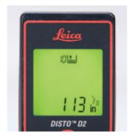
Memory. Lasers with memory store measurements even while the power is off. Nine can store the last five to 50 dimensions or results in order. The Bosch GLM 80, Stanley TLM 330, and Leica Disto E7300 and E7400x let you delete the memory so you can start a new list. Except for the Leica E7300, these also store complete calculations, as does the Spectra Precision QM55.
