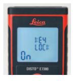
**Keypad lock.** The Stanley TLM 330 and the Leica Disto 7300 and 7400x allow you to lock the keypad. That prevents them from accidentally turning on and draining the batteries when riding in a pocket or toolbelt.
