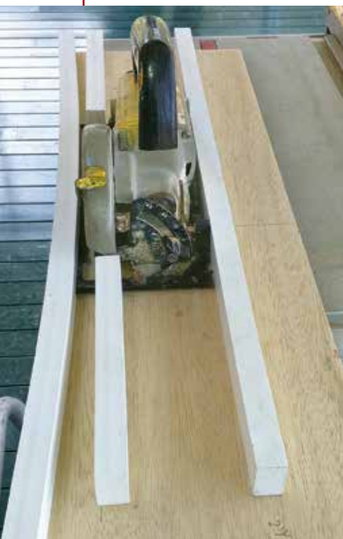
Figure 4. To cut the new decking to length after installation, the author made a plywood extension fitted with a curved fence for his Porter-Cable 4\frac{1}{2} -inch trim saw (left). One person manned the saw while another crew member removed the off-cuts (above).
