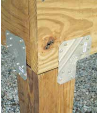
Simpson Strong-Tie LCE4 Two-piece corner connector for 4-by or 6-by lumber (new or retrofit construction)
