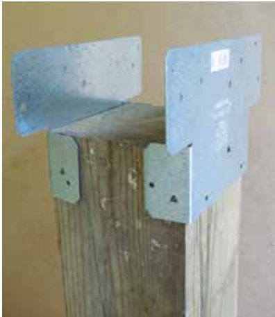
Simpson Strong-Tie AC6Z Two-piece connector for end-post installation where the sides of the post and the beam are flush (new or retrofit construction)
