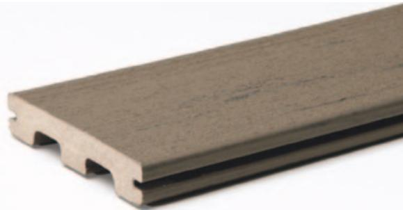
Planks come with a 25-year fade and stain warranty. They're available with a grooved profile for hidden fasteners or a solid profile that can be face-screwed, in lengths of 12, 16, and 20 feet, along with matching fascia. Boards are about 5 3/8 inches wide and 1 inch thick and span 16-inch on-center framing.
