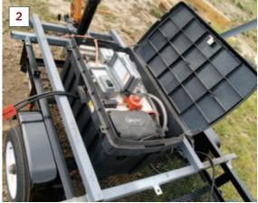
a portable unit that we could easily haul to the site and use to run our tools, and that could later be plugged into the finished structure to provide temporary power for lights and outlets (1). I don't know much about electricity, though, so I enlisted my friend and colleague Mel Wright, of Greeley, Colo., to actually put the pieces together.
