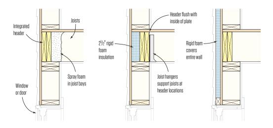
three different strategies depending on your specific situation. The first and easiest is keeping the rim joist and header even with the outside of the plate with the joists bearing on the plate, and then spraying foam insulation in each of the joist bays.
