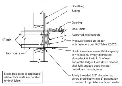
The new "permitted" lateral-load connection detail in the 2015 IRC won't require invasive interior remodeling to install, just hardware that connects the bottom of a joist back to the wall plates, foundation, studs, or window or door headers. Currently there is no widely distributed hardware for this detail, but expect to see some prior to publication of the code in early 2015. Four evenly-spaced connections are required, each of which must resist 750 pounds.
