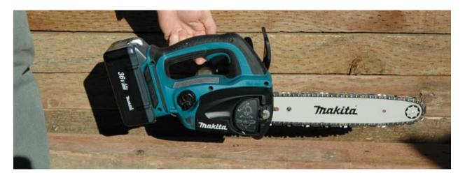
The saw can be used with either a pair of 18-volt batteries or a single 36-volt battery (shown above). The single-battery configuration offers less runtime, but better balance.
